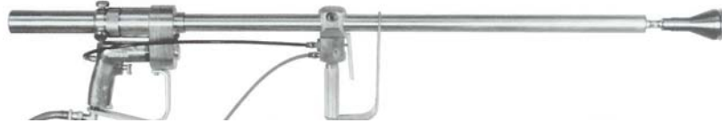
Figure 4 Pneumatically powered rotary gun, all steel/aluminium construction, driven by belt drive air motor
